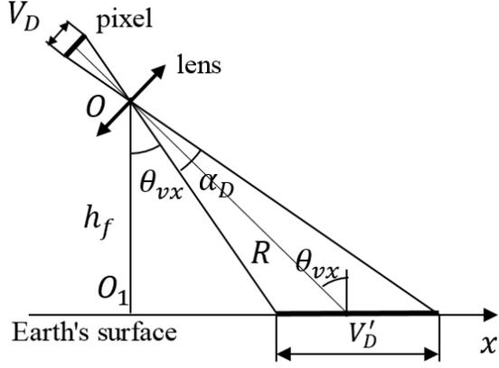
Fig. 1. Layout for ORSS spatial resolution determination
