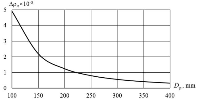
Fig. 2. Dependence of ORSS radiometric resolution on the lens entrance pupil diameter
