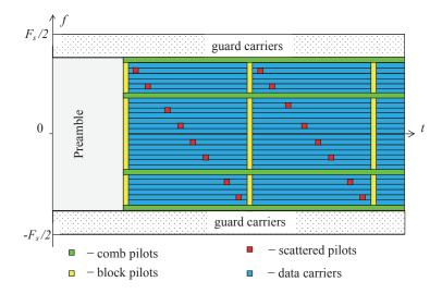
Fig. 1. OFDM signal structure in time-frequency domain
