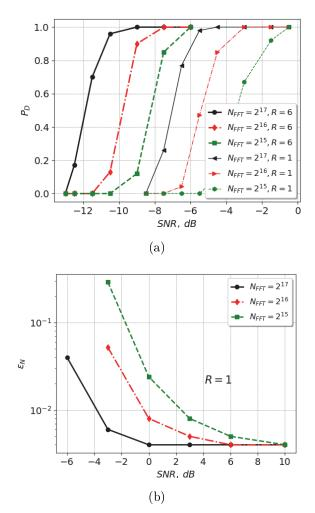
Fig. 4. Detection curves for OFDM signal (a) and relative error of frequency channels estimated number via SNR (b)
