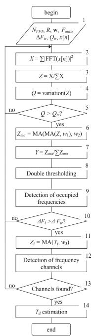
Fig. 2. Scheme of OFDM signal detection in frequency domain (MA – moving average)
