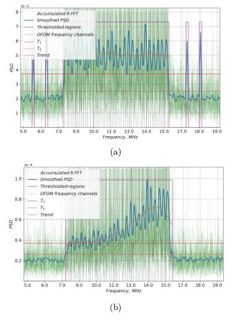
Fig. 3. Visualization of OFDM processing in fading free channel (a) and in frequency-selective channel (b)
