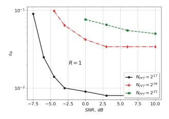
Fig. 5. Relative error of frequency channels number estimate via SNR
