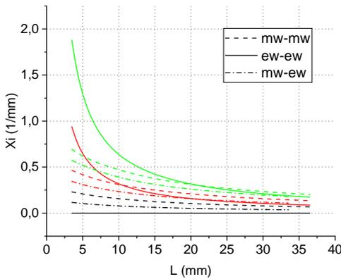
Fig. 2. Eigenvalues  $\chi_{h,n}$  of magnetic potential basic functions  $J_{h,n}$  for a strip resonator with a symmetrical open stub, obtained from the solutions of the “electrical”, “magnetic-electrical” and “magnetic” boundary value problems
