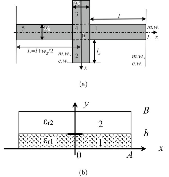
Fig. 1. Topology of a symmetrical open stub in a microstrip line (a) and cross section of a microstrip line (b)
