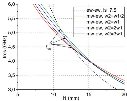
Fig. 4. The eigen frequency spectrum of a three-dimensional rectangular resonator based on a microstrip line with a symmetrical open stub, obtained from the solutions of “electrical” and “magnetic-electrical” boundary value problems with parameters (in mm):  $w_1 = 0.58$ ,  $l_s = 7.5$  depending on the stub width  $w_2$
