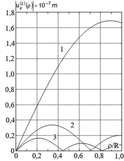
Fig. 2. Radial displacements of the piezoceramic disk material particles at the frequencies of the first three electromechanical resonances
