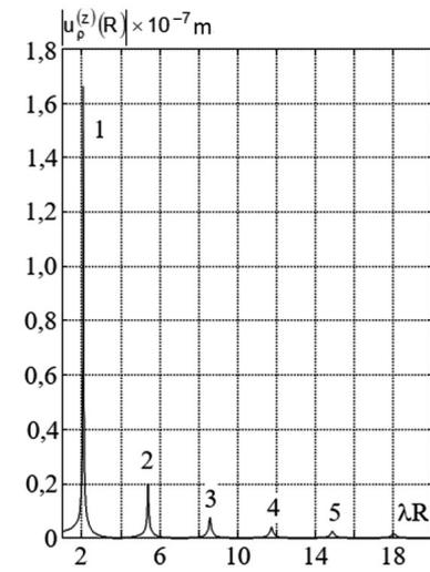
Fig. 3. Radial displacements of the piezoceramic disk's lateral surface in a wide frequency range
