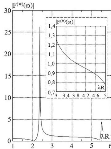
Fig. 5. Frequency-dependent alteration in the modulus of function  $F^{(*)}(\omega)$
