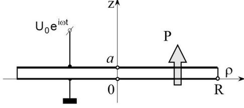
Fig. 1. Calculation diagram of a piezoceramic disk oscillating within the middle frequency range
