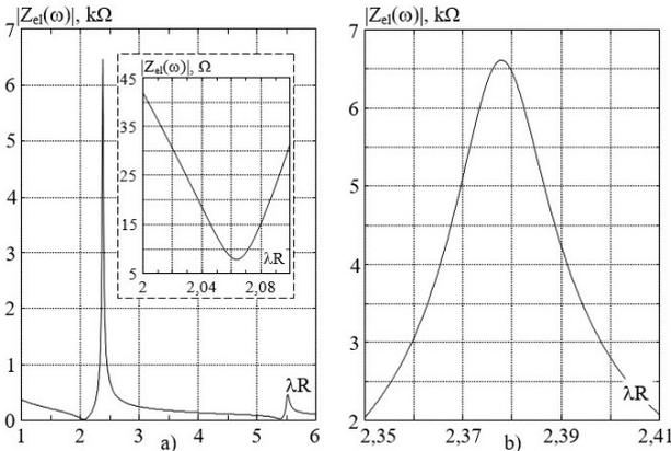
Fig. 4. Module of electrical impedance of the disk in the mid-frequency range
