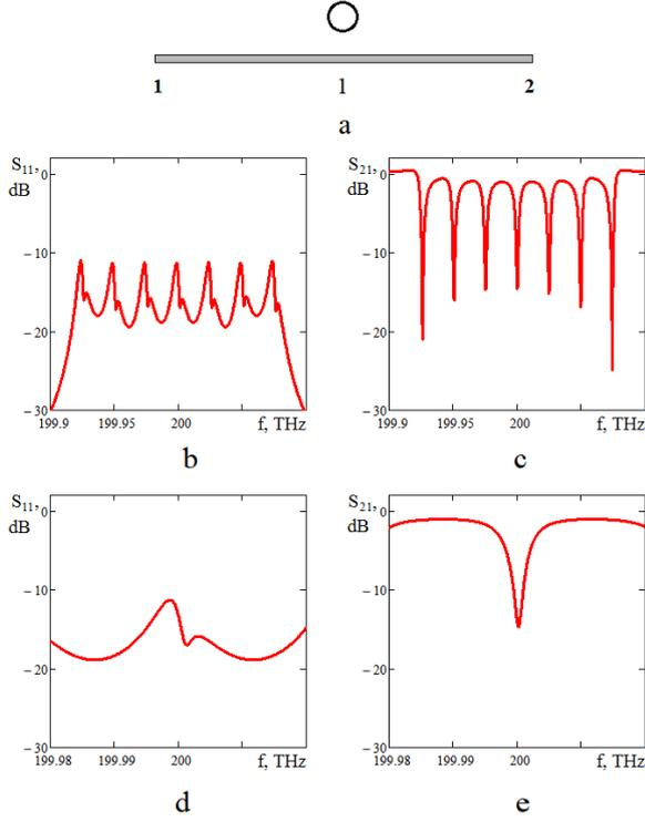
Fig. 1. Scattering characteristics (b-e) of the DR coupled with a transmission line (a) calculated for seven oscillations of WGM:  $f_0 = 200$  THz; Free Spectral Range (FSR):  $FSR = 25$  GHz; DR coupling coefficients with a transmission line: for even mode:  $\tilde{k}_s^e = 2 \cdot 10^{-5}$ , for odd mode:  $\tilde{k}_s^o = 1 \cdot 10^{-5}$ ; coupling coefficients of the resonators with open space:  $\tilde{k} = 10^{-7}$ ; dielectric loss Q-factor  $Q^D = 10^5$
