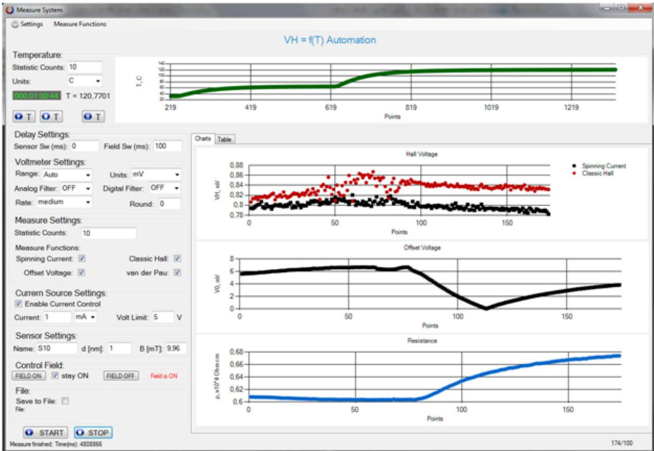
Fig. 4. Software interface of the system for measuring the temperature dependence of Hall sensor signals
