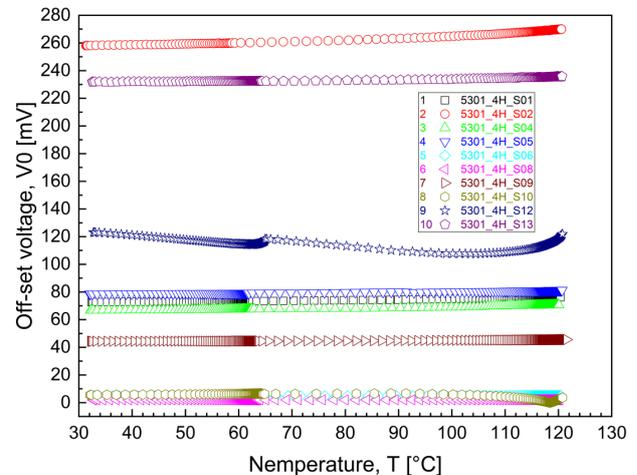
Fig. 11. Temperature dependence of the off-set signal
