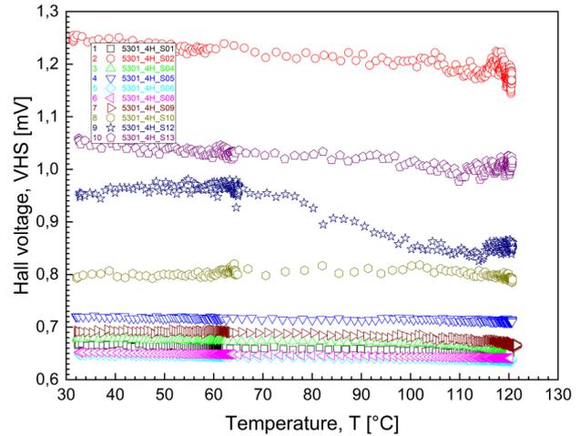
Fig. 10. Temperature dependence of the Hall signal (spinning current method)
