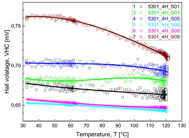
Fig. 8. Temperature dependence of the Hall signal (classical method) for samples with a small scatter
