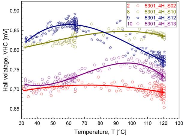
Fig. 9. Temperature dependence of the Hall signal (classical method) for samples with a relatively large scatter
