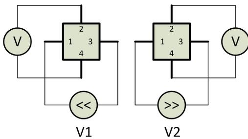
Fig. 6. Algorithm for determining the off-set signal
