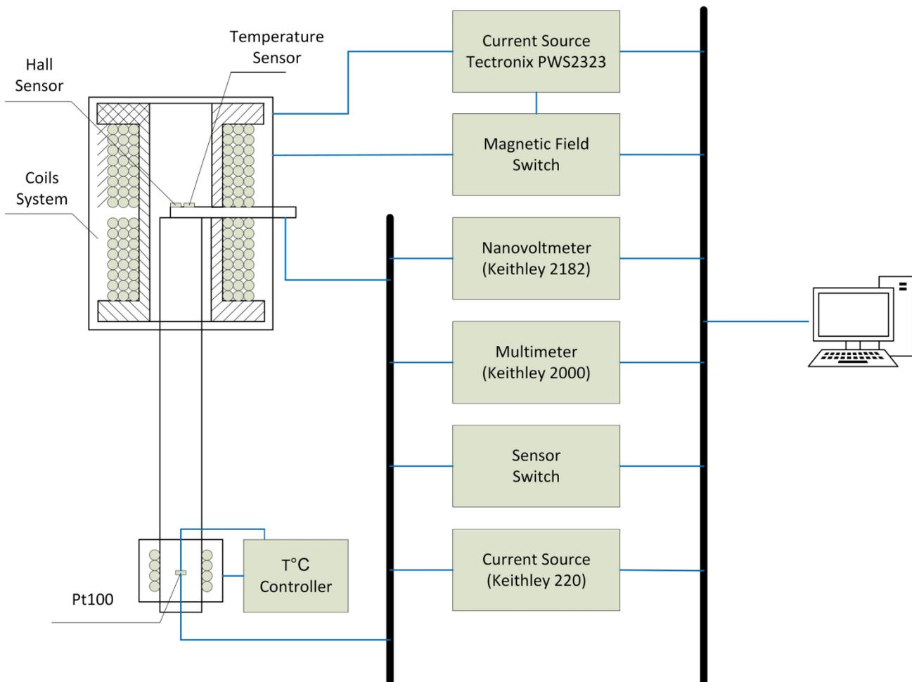
Fig. 3. Hardware of the system for measuring the temperature dependence of Hall sensor signals
