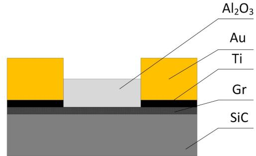
Fig. 2. Structure of the Hall sensing element
