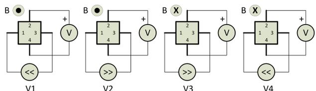
Fig. 5. Traditional method of extraction the Hall signal
