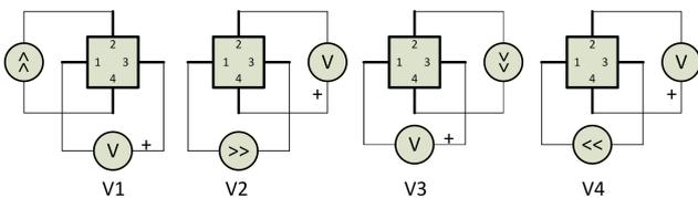
Fig. 7. Spinning current algorithm
