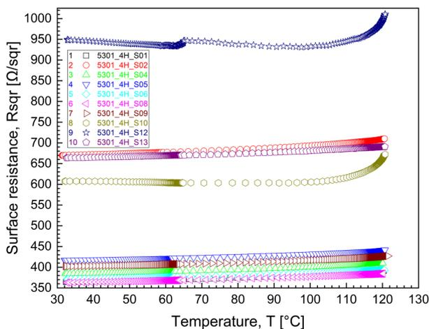
Fig. 12. Temperature dependence of surface resistance
