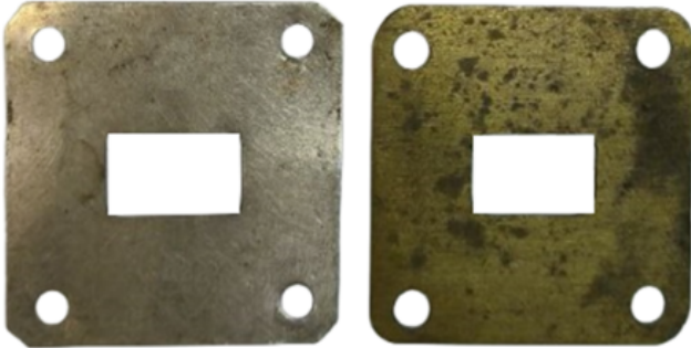
Fig. 4. Inductive irises used in measurements
